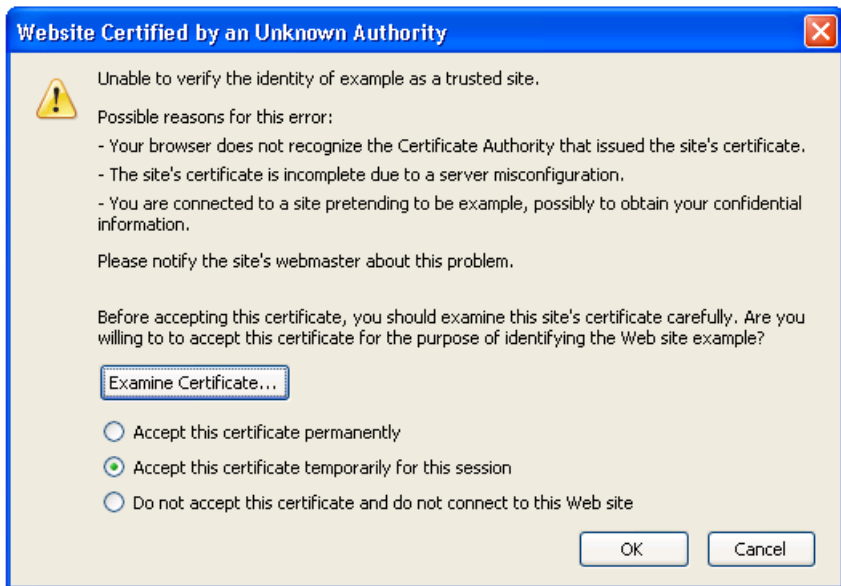
Fig. 2. Mozilla Firefox warning that a certificate is not signed by a trusted CA
